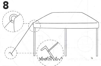
Use the guy ropes attached to the ring at each corner of the roof cover and stakes, to secure your Pop-Up Gazebo to the ground or just use the stakes through the hole in each leg foot.
