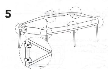
Place the cover over frame. Attach the Velcro tabs, located on the underside of the top cover, around the frame struts.
