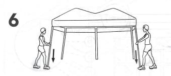
You and your partner should each place a foot on the foot plate of the bottom of adjacent legs and lift up the leg, sliding the inner leg out until the snap button locks in the locating hole. Repeat this operation for the other legs.
