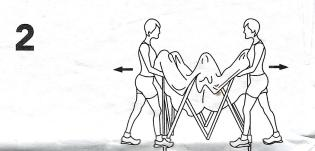
With your partner on the opposite side, grasp two outer legs, slightly lift the frame off the ground and take a small step backwards. Be careful not to pull backwards too hard as this will result in the side supports bending.
