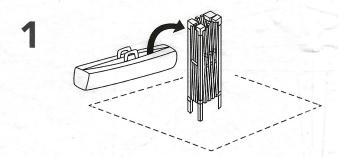
Place your Pop-Up Gazebo in the centre of the area to be sheltered. Remove the carry bag and stand the Gazebo on its feet. Check to make sure that the roof struts are not stuck before moving.
