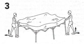
Push the top and bottom of the diamond formed by side supports together. Then move to the opposite corner and do the same, move from one corner pole to the other taking a small step backwards each time until the Gazebo is almost fully open.
